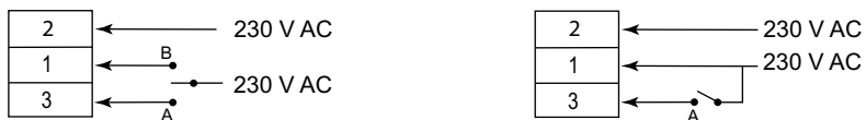
Fig. 4 Left = 3-point, Right = 2-point; 1 = Black; 2 = White; 3 = Red; A = Actuator stem extend; B = Actuator stem retract
