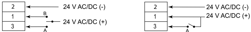
Fig. 3 Left = 3-point; Right = 2-point; 1 = Black; 2 = White; 3 = Red; A = Actuator stem extend; B = Actuator stem retract
