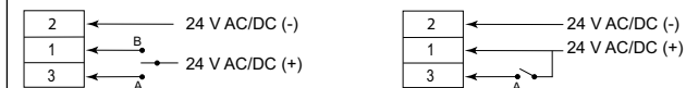
Figure 2 Left = 3-point; Right = 2-point; 1 = Black; 2 = White; 3 = Red; A = Actuator stem extend; B = Actuator stem retract
