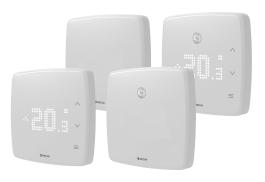
Regio RCX series are controllers with built-in sensors and an RS485 communication port. Controllers in different rooms and zones can be connected to a field bus enabling communication with a central SCADA system, via RS485 (EXOline, BACnet, or Modbus). They can also be used as stand-alone controllers for control of heating and cooling in a single zone or room.
