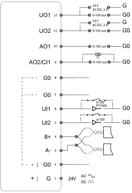
Fig. 2 General wiring example
