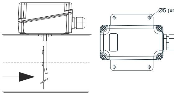
If the duct is vertical, the range of the flow switch must be recalibrated so that the paddle weight is properly balanced.
