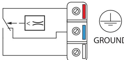
Connect to the red and white contacts of the microswitch. They will open when the flow drops below the set level.
