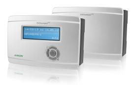
EXOcompact Vido is a 230 V AC freely programmable controller especially suitable for heating applications. It provides built-in communication via EXOline, Modbus or BACnet for integration into EXOscada or other SCADA systems. It can be used either as a stand-alone unit or as part of a larger system.
