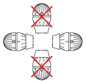
In order to prevent inaccurate temperature readings, the thermostat should be installed in a place with a representative room temperature, for example not exposed to direct sunlight, or in a cold draught.
