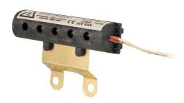
Valve stem heater to be used in systems with media temperatures below 0 °C to prevent freezing and blockage from ice formation. Can be used with all valves when RVAN-actuator is used.
