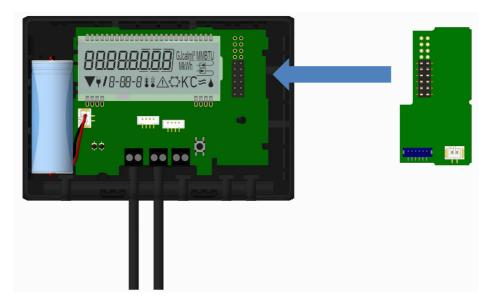
To remove a module the upper housing piece must be carefully pressed against the rear panel of the lower housing piece during opening the calculator. Thus the two rear snap-fits of the upper housing piece lever out the module of the PC board (see picture 4).
