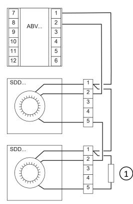
Fig. I Wiring SDD-S65-OE to ABV... Note: -RAC models should not be mounted in loop or to a control unit
