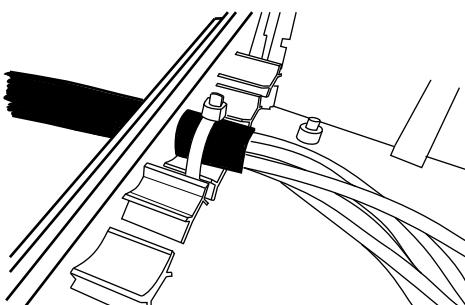
Figure 2 Secure the cable with a cable tie
