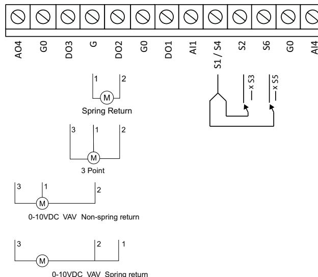
Figure 5 Actuators and end position switches
