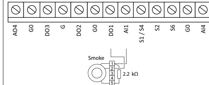
Figure 6 Smoke detector connected to power and Analogue input 1
