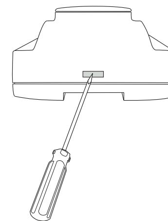
Figure 6 Removing the top of the casing.
