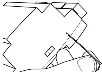
Figure 4 Resetting the application memory.
