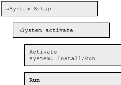
1. Go to **System setup** in the main menu in the master unit by using [▼].
