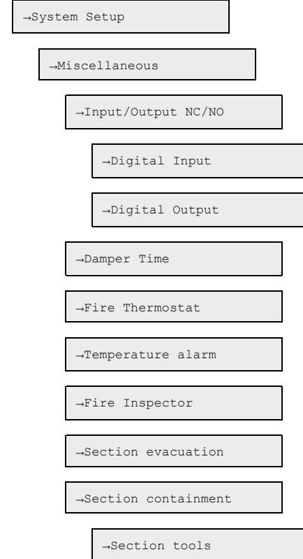
Use the [OK], [►], [▼], and [▲] buttons for miscellaneous system setup functions. Here you can change input and output (only view of values), damper time, fire thermostat, temperature alarm (see separate procedure *Setting master unit temperature alarm*), fire inspector, section evacuation, and section containment (see *Sections*.)
