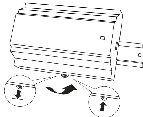
Figure 5 Removing the controller from the DIN rail.
