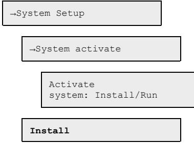
1. Go to **System setup** in the main menu in the master unit by using [▼].
