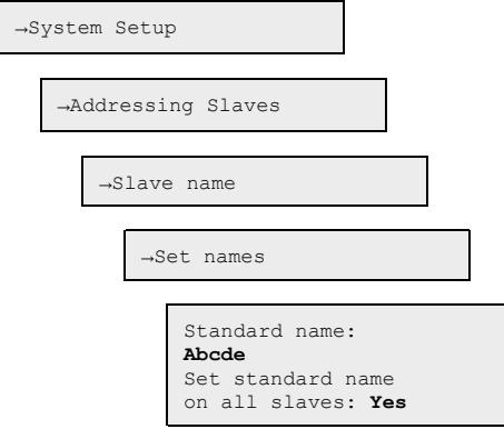
1. Go to **System setup** in the main menu in the master unit by using [▼].
