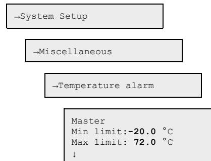
1. Go to **System setup** in the main menu in the master unit by using [▼].
