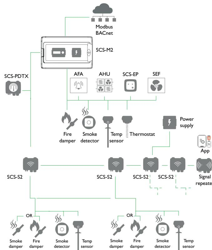
Figure 1 System setup example
