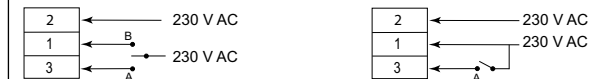
Figure 2 Left = 3-point, Right = 2-point; 1 = Black; 2 = White; 3 = Red; A = Actuator stem extend; B = Actuator stem retract
