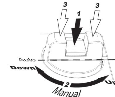
To manually set the valve position, first depress the central part of the knob, until it clicks and remains depressed (1 in the figure). Then the valve position can be changed manually by turning the knob (2 in the figure). When the knob is turned clockwise, the drive rod is pushed outwards and when the knob is turned anti-clockwise, the drive rod is pulled inwards.
