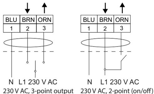
\*\*PCTV, PCTMV and PCTVS DN15-32 valves are normally open. They close when the actuator stem extends.
