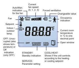
It is possible to set different parameter values in a parameter menu in the display, using the buttons on the controller. You change parameter values with the INCREASE and DECREASE buttons and confirm changes with the Occupancy button.
