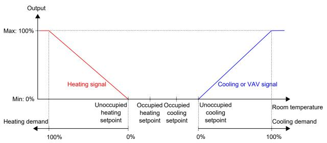
Figure 3-26 Control behaviour for the unoccupied controller state.
