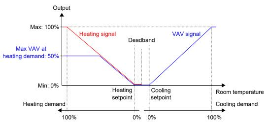
Figure 3-40 Control behaviour for the Heating + VAV controller mode when the maximum VAV output on heating demand setting is applied.
