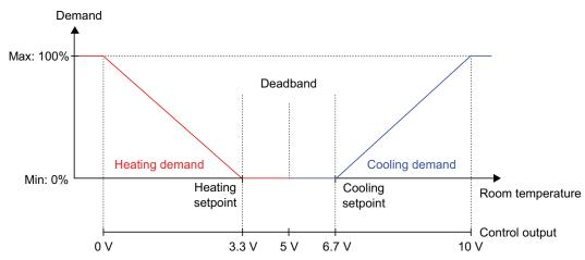
Figure 3-45 Simplified view of an AO configured for the 6-way valve with the controller in controller mode Heating + Cooling + VAV
