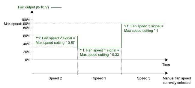
Figure 3-33 EC fan control behaviour in manual mode (fan speed 1, 2, or 3).
