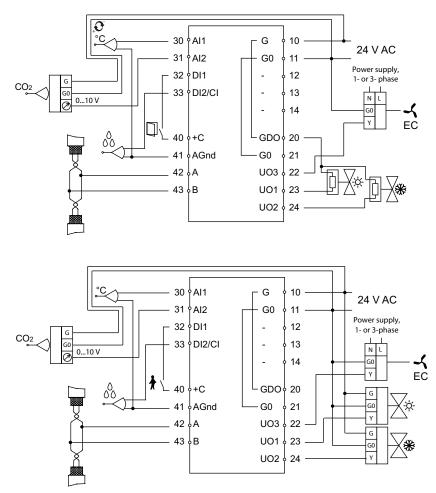
Figure 6-5 Connection diagrams for models for CO2 control and fan control.
