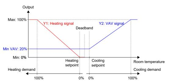
Figure 3-10 Control behaviour for the Heating + VAV controller mode when the controller regulates based on heating and cooling demand.
