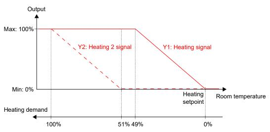
Figure 3-3 Control behaviour for the Heating + Heating controller mode.
