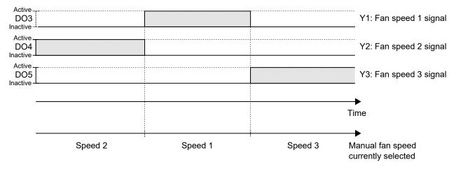
Figure 3-36 3-speed fan control behaviour in manual mode (fan speed 1, 2, or 3).
