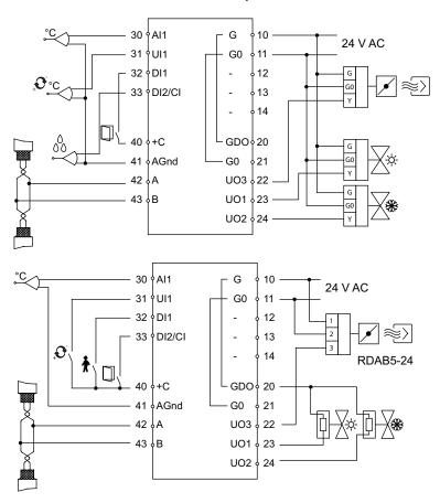
Figure 6-2 Connection diagrams for basic models with 3 universal outputs.
