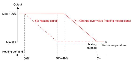
Figure 3-12 Control behaviour for the Heating + Heating/Cooling (change-over) controller mode when the controller is in Heating + Heating mode.
