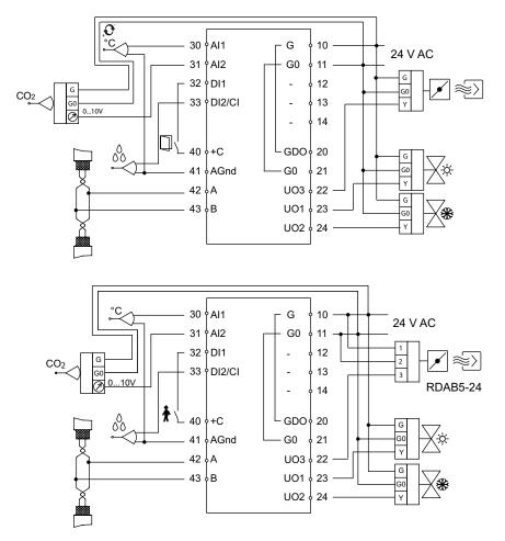
Figure 6-3 Connection diagrams for model for CO2 control.
