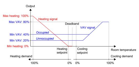
Figure 3-39 VAV control behaviour based on cooling demand when a maximum limit is set, and minimum limits for the occupied and unoccupied controller states are set.
