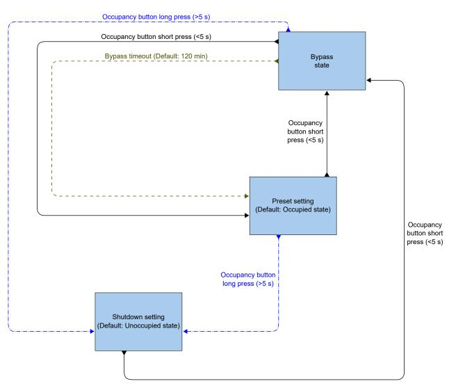
Figure 3-29 Flow chart describing controller state changes for when the occupancy (on/off) button on the controller is used.
