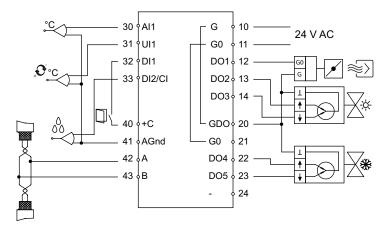
Figure 6-7 Connection diagrams for models for three-point control.
