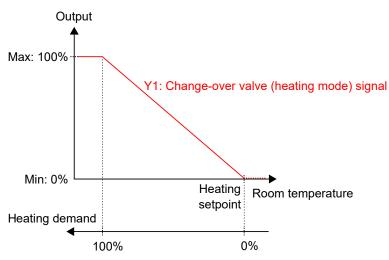
Figure 3-14 Control behaviour for the Heating/Cooling (change-over) controller mode when the controller is in heating mode.
