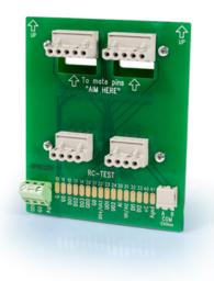
In order to make measurements and test the inputs/outputs of a Regio room controller during installation, Regin's RC-TEST service adapter may be used.
