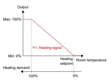
Figure 3-2 Control behaviour for the Heating controller mode.
