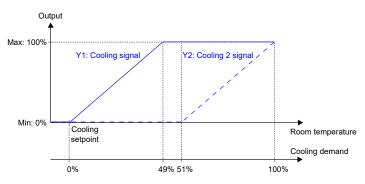
Figure 3-6 Control behaviour for the Cooling + Cooling controller mode.
