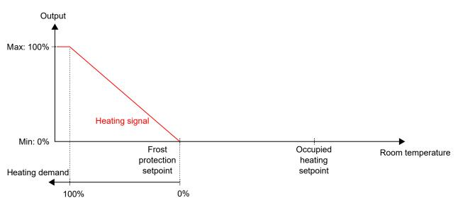
Figure 3-25 Control behaviour for the off controller state.
