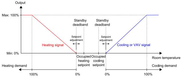
*Figure 3-27* illustrates the control behaviour when no maximum or minimum limits are set for the output signals.
