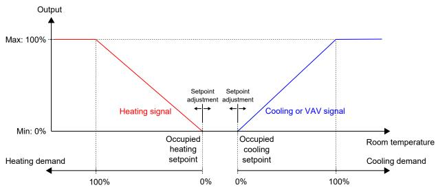
Figure 3-28 Control behaviour for the occupied and bypass controller state.
