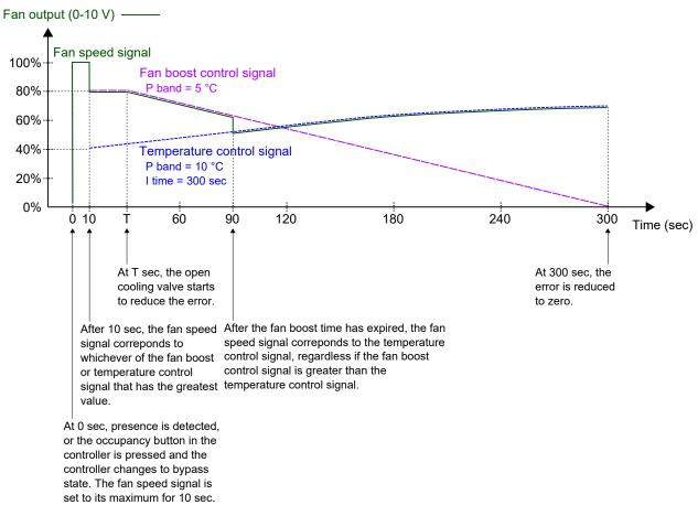
Figure 3-37 An example of fan boost control behaviour for an EC fan in auto mode, which provides a perceived cooling effect until the cooling distribution from the cooling valve establishes. The P-band for the fan boost controller has a lower value (higher gain) than the P-band for the temperature controller.
