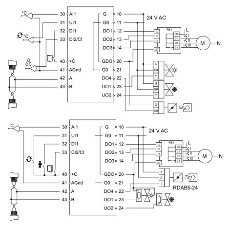
Figure 6-6 Connection diagrams for models for fan control.
