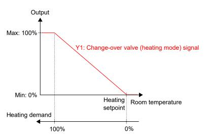
Figure 3-7 Control behaviour for the Heating/Cooling (change-over) controller mode when the controller is in heating mode.
