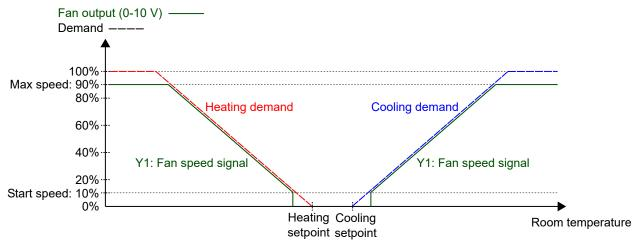
Figure 3-32 EC fan control behaviour in auto mode.
