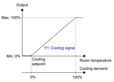
Figure 3-5 Control behaviour for the Cooling controller mode.
