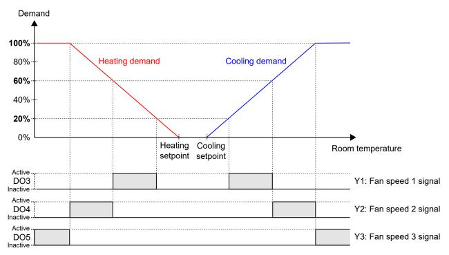
Figure 3-35 3-speed fan control behaviour in auto mode.
