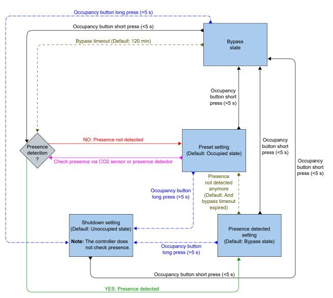
Figure 3-30 Flow chart describing controller state changes for when presence detection and the occupancy (on/off) button on the controller is used.
