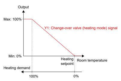
Figure 3-19 Control behaviour for the Heating/Cooling (change-over) controller mode when the controller is in heating mode.
