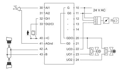
Figure 6-4 Connection diagrams for model with built-in CO2 sensor.
