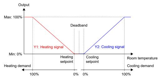
Figure 3-4 Control behaviour for the Heating + Cooling controller mode.
