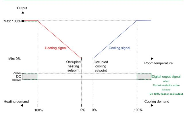
Figure 3-42 Example of forced ventilation control behaviour for the Heating + VAV controller mode when the controller is in bypass state.
