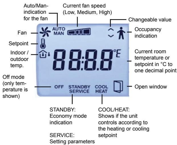
The display is handled using the buttons on the controller:
