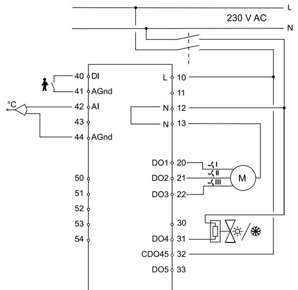
Wiring diagram for thermal actuator
