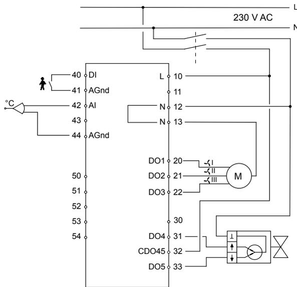
Wiring diagram for 3-point actuator
