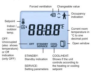
The buttons on the controller enables easy setting of parameter values using a parameter menu shown in the display. The parameter values are changed with the INCREASE and DECREASE buttons and changes confirmed with the occupancy button.
