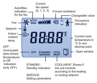
The buttons on the controller enables easy setting of parameter values using a parameter menu shown in the display. The parameter values are changed with the INCREASE and DECREASE buttons and changes confirmed with the occupancy button.
