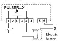
U: Outputs for wiring of PULSER-ADD
