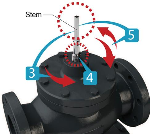
3. Remove the actuator and actuator assembly and then loosen the stem completely by turning it anti-clockwise
