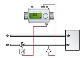
The AO1 output signal will increase when the pressure signal falls below the setpoint value.
