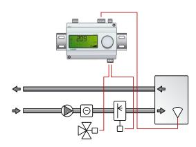
AO1 and AO2 are controlled in sequence. A neutral zone for the controller can be set between AO1 and AO2. The actual value must be provided by a transmitter with an output signal of 0...10V DC. This control mode can for instance be used for humidity control. If so, use one of the below Regin brand sensors:
