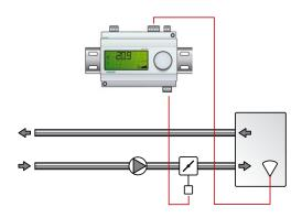
The output signal will increase when the CO<sub>2</sub> value rises above the setpoint value.
