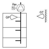
The output signal will increase when the pressure signal falls below the setpoint value.
