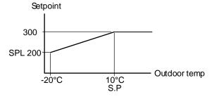
Example: With an ordinary setpoint of 300 Pa, a starting point S.P of  $+10^{\circ}$ C and a SPL of 200 Pa at  $-20^{\circ}$ C you get the following setpoint-to-outdoor temperature relation
