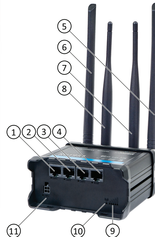
Figure 1 Router connections and antennas
