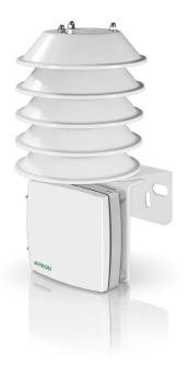
HVS is a weather shield for outdoor mounting of Regin's HTWT10 and HTWT10-420 transmitters. The weather shield is designed so as to create air circulation around the sensor element, thereby ventilating it to prevent overheating during strong sunlight.
