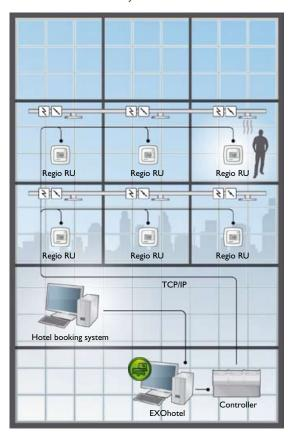
When the hotel guest checks in, a message is sent from the booking system to EXOhotel, which in turn sends a command to the controller in the guest room to go to economy mode. When the guest arrives at the room and puts the keycard in the reader, the running mode switches to comfort mode with forced ventilation. When the guest
