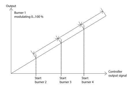
When boiler 1 is configured to a digital function (1-step or 2-step) the digital outputs will step into sequence by one step at a time, and each time a digital output is switched on or off the controller will be blocked for the set time period (see picture below).
