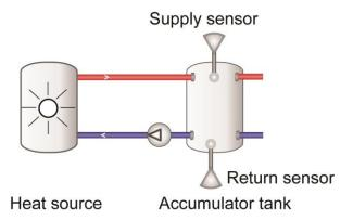
Loading is started if the return water temperature is lower than the set start temperature.
