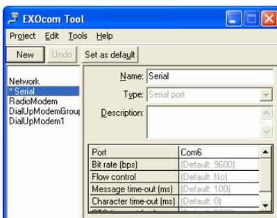
Check that the suggested Com port corresponds to the Com port which the computer has assigned to E-cable. You can see which Com port has been assigned in the Control panel / System / Device Manager / Ports (COM & LPT).
