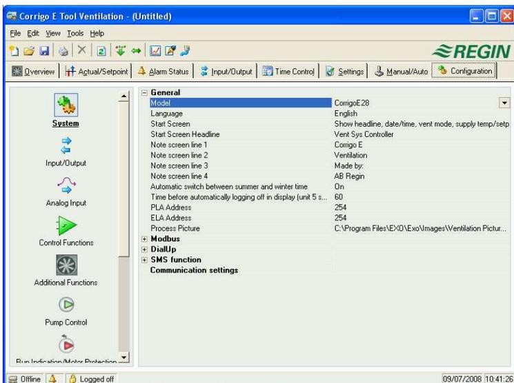
This folder contains all the configuration parameters for the Corrigo. Since the contents are very diverse, the folder has been divided into sub-folders. These are accessed by clicking on the buttons in the left-hand button-list. For detailed information on these, please see the manual for the controller in question.
