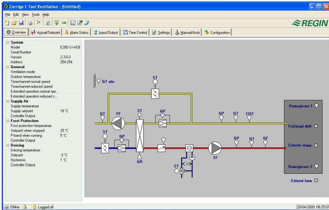
The major part of the Overview folder displays a process diagram. The diagram is a static bitmap illustration that can be edited using, for example Paint. Any number of different diagrams can be saved. Which diagram is displayed is governed by the setting of the parameter *Process picture* in the System sub-folder in the Configuration folder.
