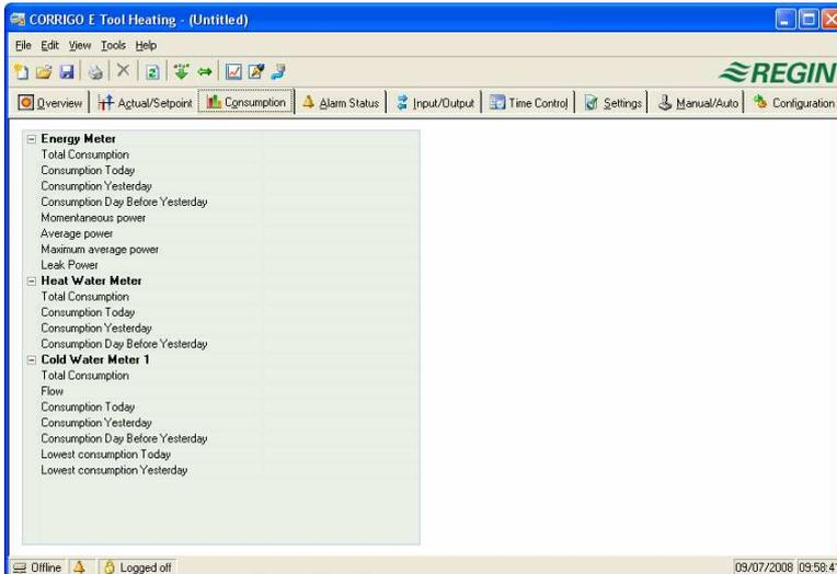
Displays consumption values for Energy Meter, Heat Water Meter and Cold Water Meter. The values are calculated using pulse constants that are set in the submenu Pulse constants in the Configuration folder.
