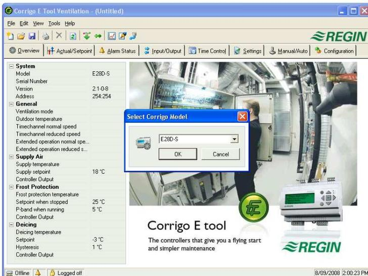
E tool always starts with a box where you enter which Corrigo model you are using. The Overview folder is also displayed. Make sure that you enter the correct model, or strange things may occur in the control and alarm handling.
