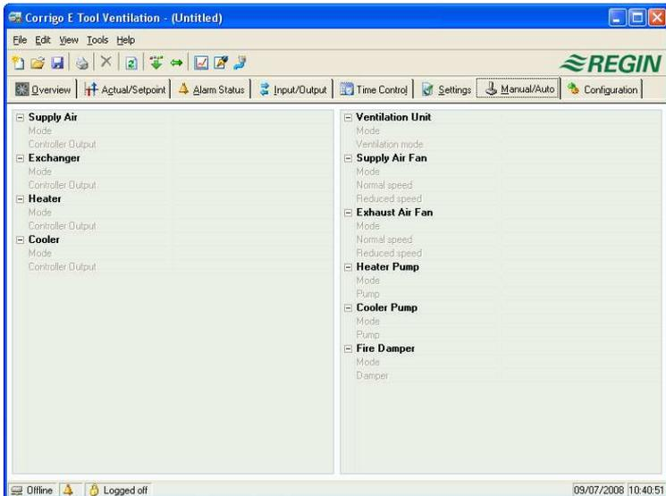
In this menu you can take manual command of most controller functions. Very useful for testing purposes.
