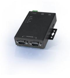
E-BACNET2-V is a pre-configured converter for connecting a Corrigo E running a ventilation application to a SCADA system via BACnet. Communication with the Corrigo E takes place via EXOline RS485 and is pre-set to PLA:ELA address 254:254, meaning that in most cases it is possible to connect directly without changing any settings in the Corrigo E. Communication between the converter and the SCADA system takes place via BACnet/IP. The unit is supplied with cables and a power adapter.
