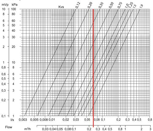
The valves have adjustable kvs value (kvs = the flow in m³/h at a pressure drop of 100 kPa).
