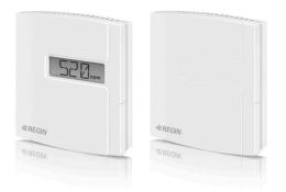
A range of room transmitters for measuring carbon dioxide concentration in indoor environments. The transmitter has a built-in  $CO_2$  sensor with working range 0...2000 ppm, as well as a built-in temperature sensor.
