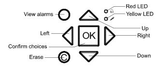
There are seven buttons: four arrow buttons which will be called UP, DOWN, RIGHT and LEFT. The menus in the Corrigo E are organized in a horizontal tree structure. The UP/DOWN buttons are used to move between menus at the present menu level. The RIGHT/LEFT buttons are used to move between menu levels. When changing parameters the UP/DOWN buttons are used to increase/decrease the value of the parameter and the RIGHT/LEFT buttons to move between digits within the parameter.
