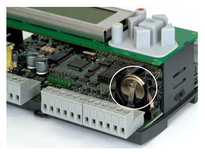
Grip the battery firmly with your fingers and lift it upwards until it rises from its holder.
