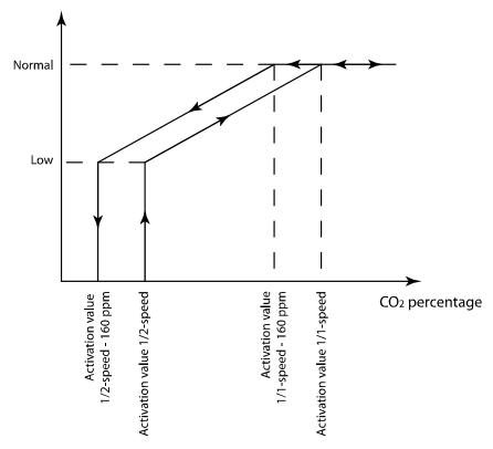
When used with 2-speed fans they will start using reduced speed when the  $CO_2/VOC$ -value rises above control value one and switch to normal speed when the  $CO_2/VOC$ -value reaches control value two. The fans will stop when the  $CO_2/VOC$ -value falls 160 ppm below control value one.
