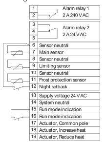
The common terminal on the actuator must be connected to output common, terminal 17, on the controller.
